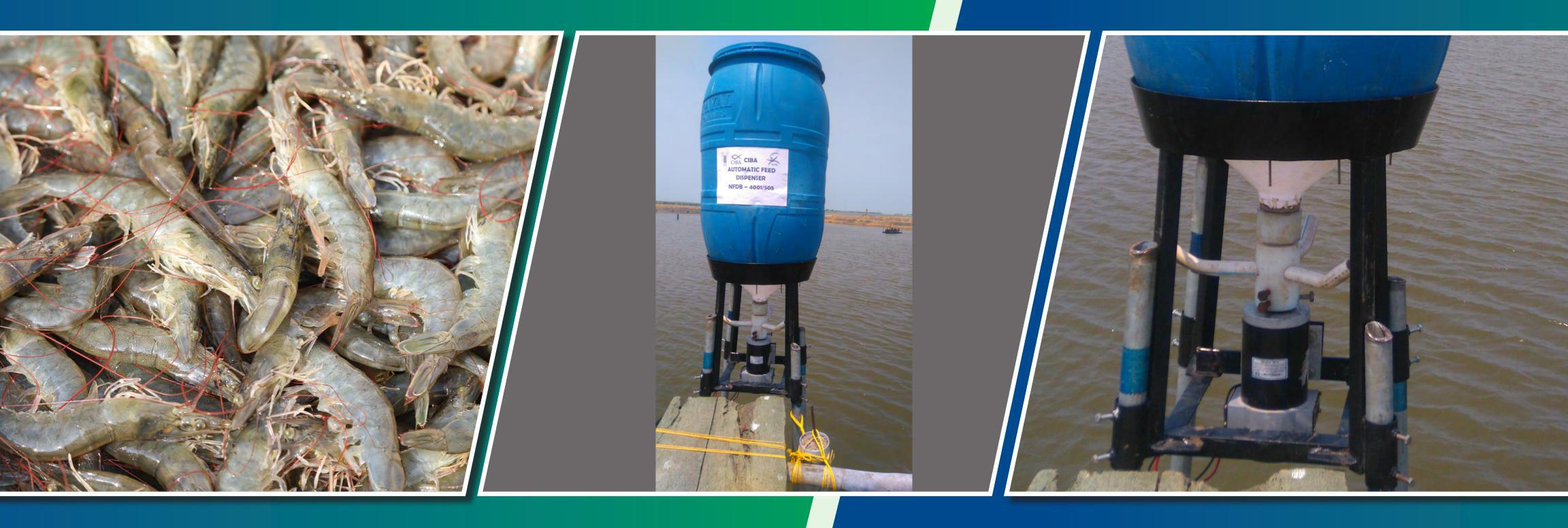
Solar-powered automatic feeders are designed to dispense feed at pre-programmed intervals. This automation ensures that animals receive their feed consistently, even when technicians are away or occupied with other tasks. It's particularly important for shrimp culture especially in *P. vannamei*, as it can help maintain regular feeding schedules.
