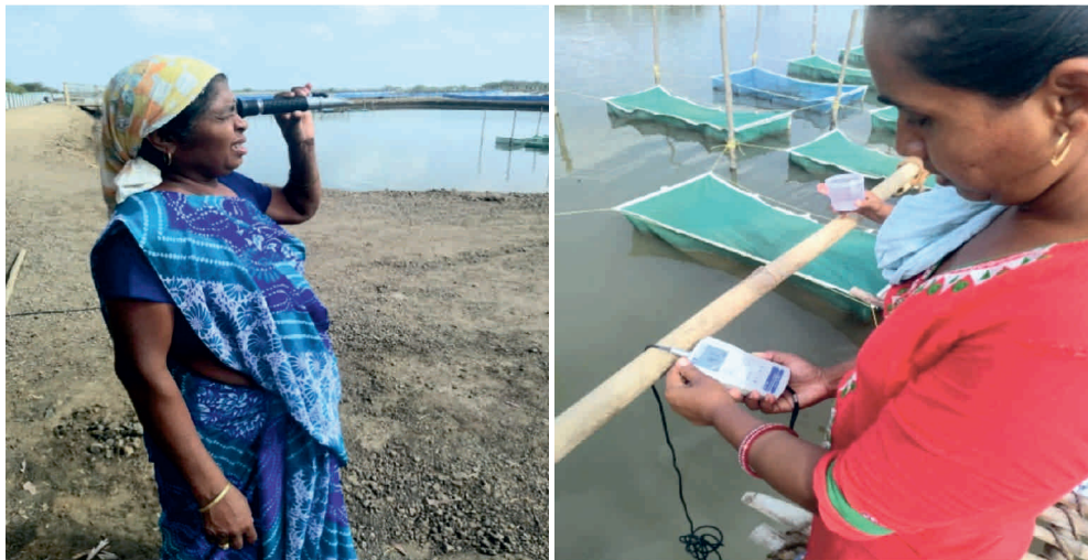
Monitoring of seabass nursery pond water salinity and dissolved oxygen
